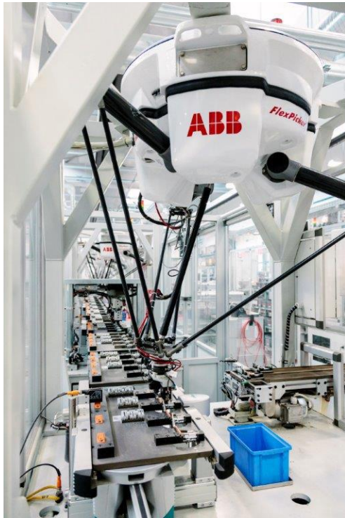
The Flexpicker from ABB: Highspeed-Picking at electronics production
